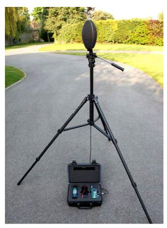
The Castle Weatherproof Sound Meter enclosure is designed to make short- to medium-term outdoor noise monitoring simple and effective. Dedicated to the Castle SONUS 'L' or 'E' Data-logging sound meters, this box opens up a huge range of possibilities for longer term monitoring both indoors and out. And what is more, it weighs less that 5Kg's, so is one of the lightest environmental noise monitors in the world!
